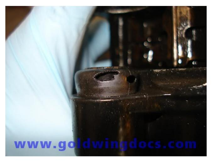
18. The pivot bolt is dirty. Clean any dirt and corrosion gently, then polish with sandpaper the same way you polished the pistons. Careful, it is very soft aluminum.
