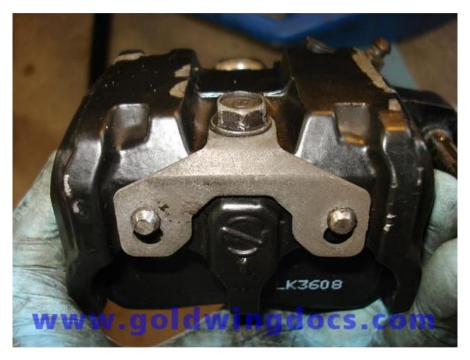
32. Apply high-temperature brake lubricant to the pivot bolt. You may have to remove this bolt before the caliper is replaced on some models.
