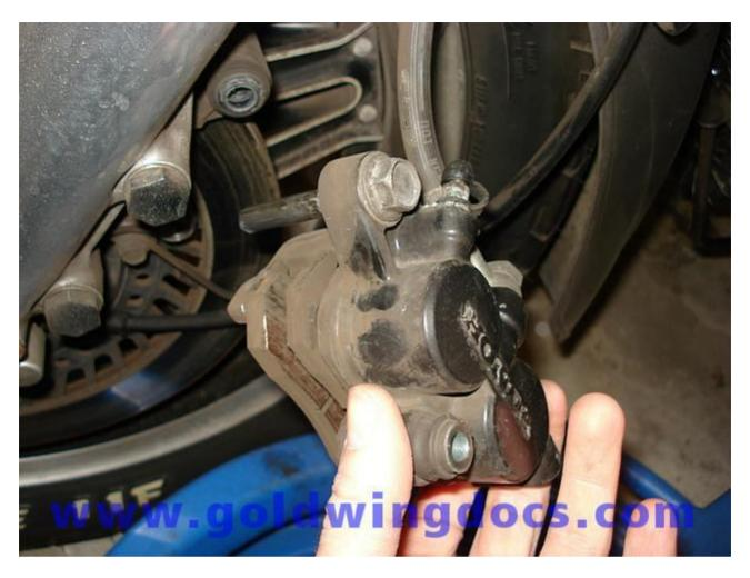
3. Unbolt the brake pin retainer bracket bolt.
