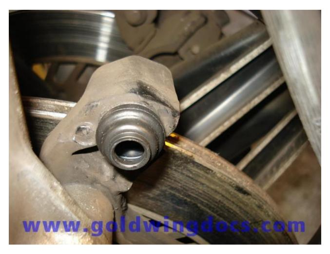
29. Insert the retainer spring into the caliper.
