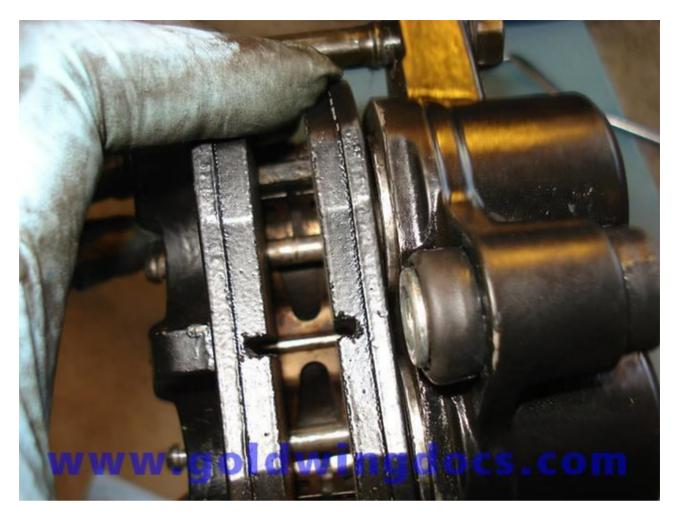
31. Place the brake pin retaining bracket in place, and fasten the bracket retaining bolt.
