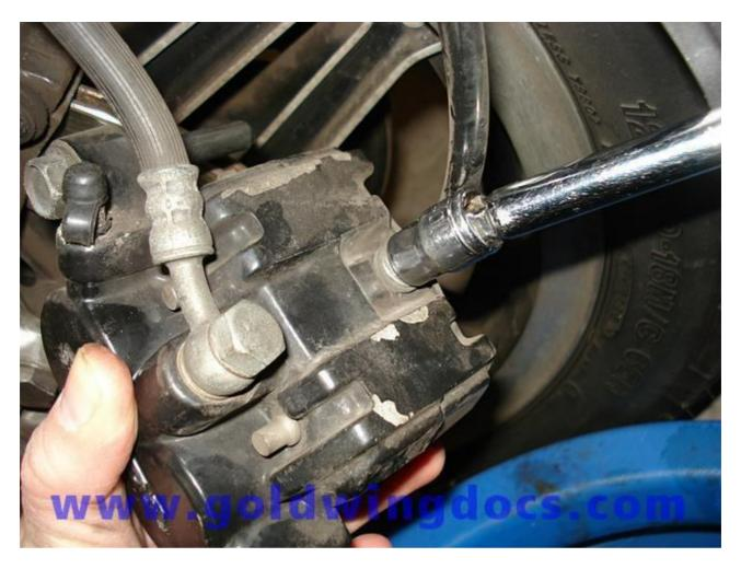
4. Remove the brake pin retainer bracket.
