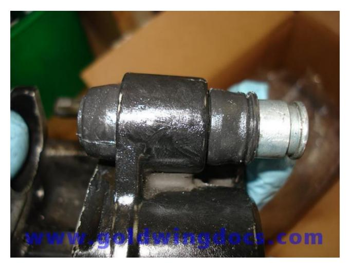
27. Remove the boot from the pivot receptacle on the fork leg, and clean the inside of the receptacle with brake cleaner.
