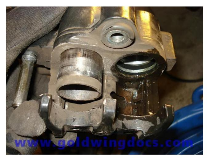
12. Remove the banjo bolt fitting holding the brake line to the caliper.
