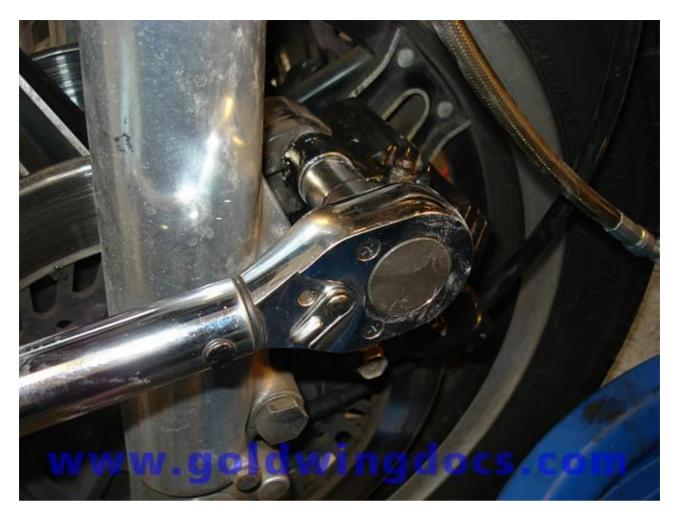
35. Replace the banjo bolt on the brake line fitting, using new crush washers on either side of the banjo.
