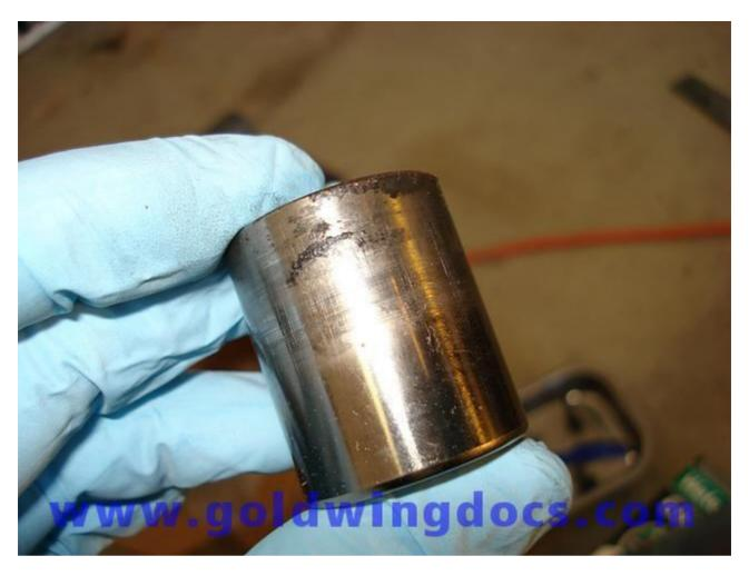
16. Polish in a circular motion (never in a straight line) first with the 600 grit sandpaper, then with the 1500 grit sandpaper to polish it. After polishing with the 1500 paper, this is what it should look like - it will be extremely smooth to the touch.
