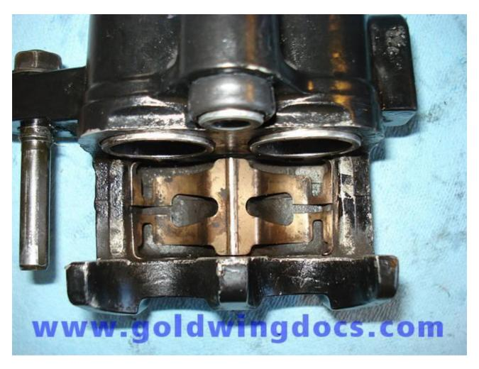
30. Push the new brake pads into the caliper, then push the brake pad retaining pins through to hold them in place.
