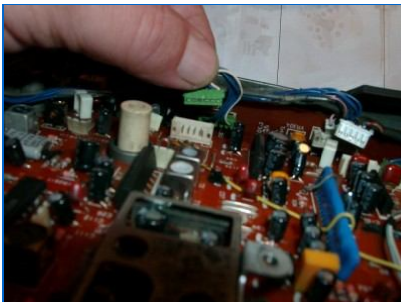
REMOVING THE CONNECTORS
