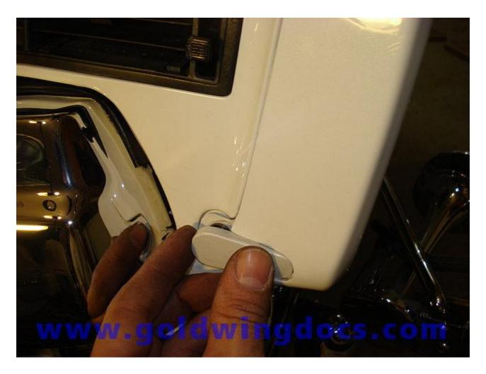
10. Be very careful removing these covers - pulling them back too far will snap the tab off of the outer edge. See how the tab hooks into the cowl. Gently rotate the inner edge back, then pull it straight out.
