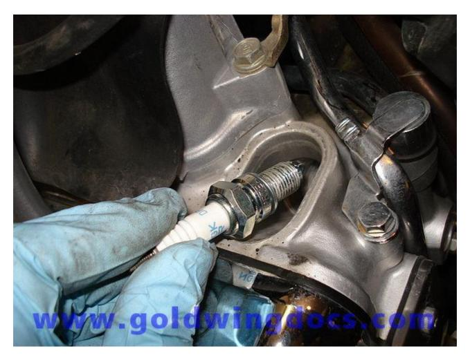
26. Place the spark plug socket over the plug and continue to thread it in by hand until it is finger-tight.
