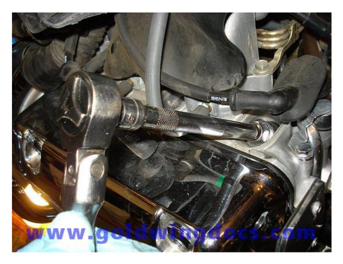
21. New spark plugs should be gapped to 0.031 to 0.035 inches - although it has been a long time since I saw new plugs from the manufacturer that weren't already gapped correctly.
