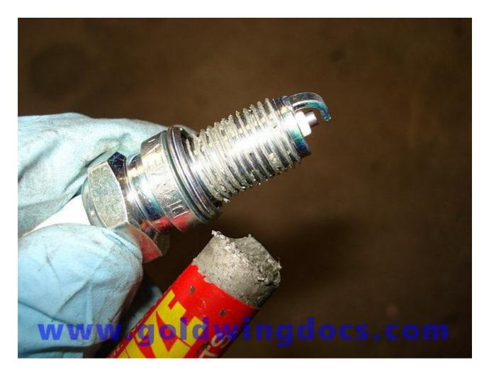
25. Insert the spark plug into the well and start threading it in by hand until you are sure it is not cross-threaded. Cross-threading a plug in an aluminum head has dire consequences!
