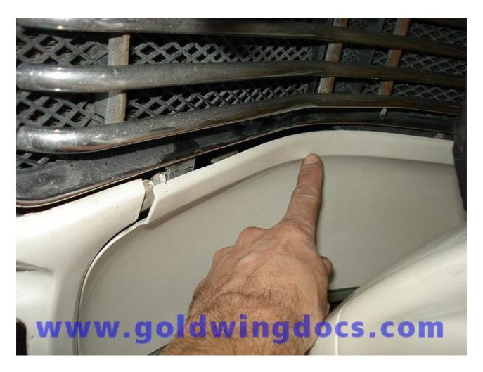
4. Gently pull the top corners away, one at a time, to unseat the posts from their grommets. Note the black tab that is holding the front of the lower cowl in place - it's important that the lower cowl is fitted back behind these tabs when it is replaced.
