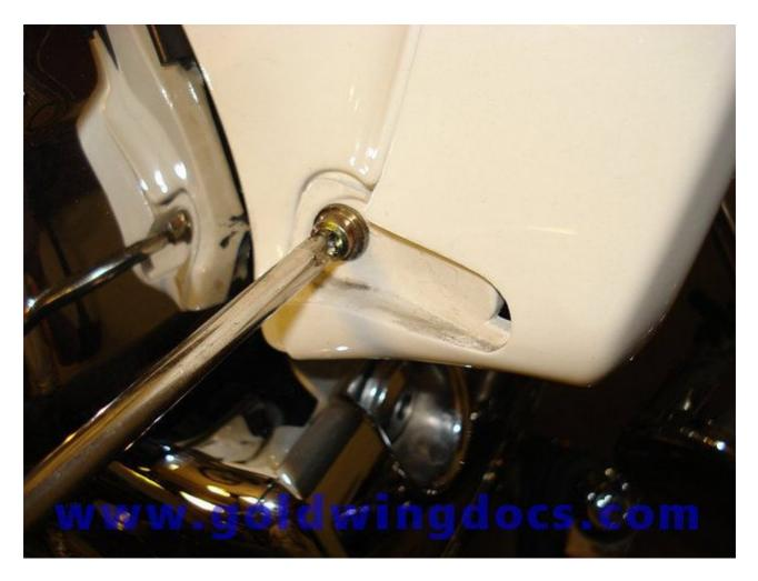
12. Gently remove the lower cowl deflector. It pulls out approximately one inch at the bottom, then is pulled straight down to disengage the top tab, then is pulled straight back to disengage the front tab.
