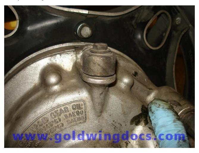
That is a vent. As it heats up in there (and it does get warm), the air needs a place to escape, so it doesn't blow out the seals. Similarly, air needs to get back in once it cools off.
