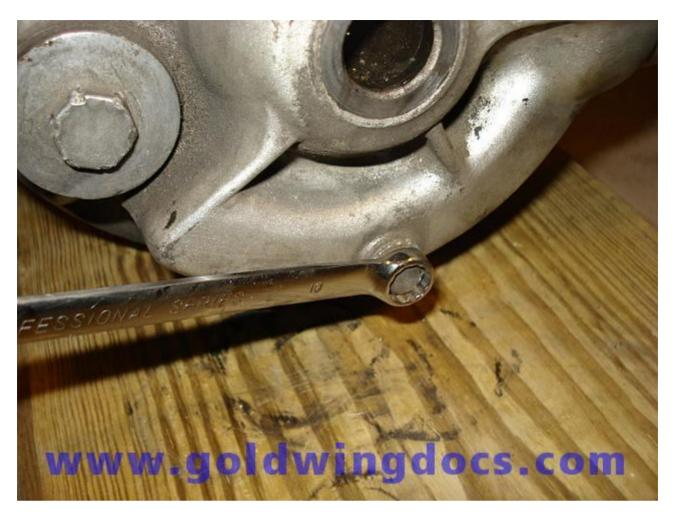
3. After all the gear oil has drained, replace the drain plug, and remove the fill plug.
